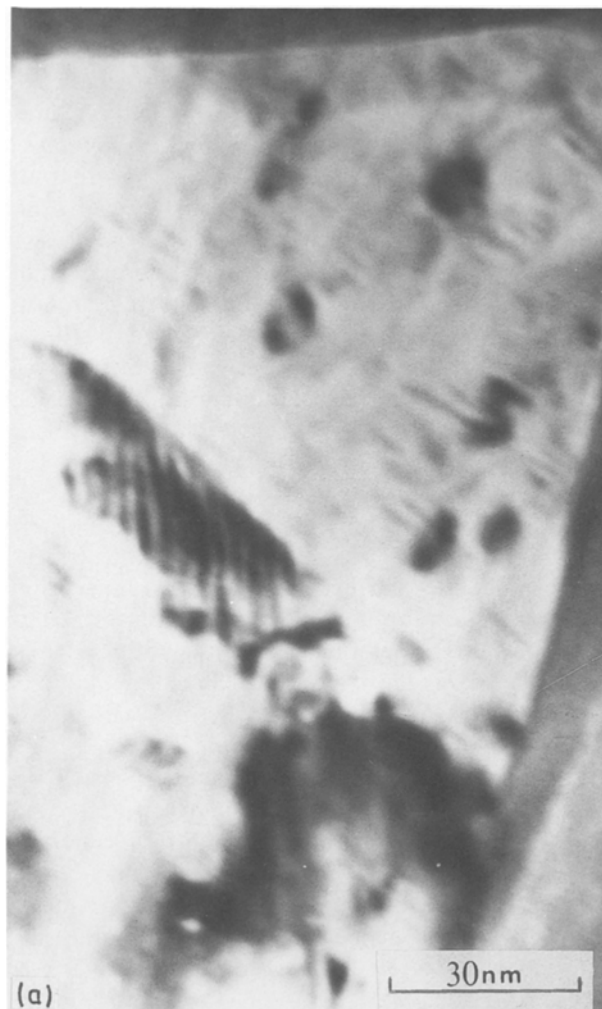
Figure 8 (a) Bright-field micrograph of a Pb-rich second-phase inclusion at a triple junction. The dark patches of contrast present in the micrograph originate from the effects of electron-beam irradiation. (b) SADP corresponding to the second-phase inclusion of Fig. 8a.
