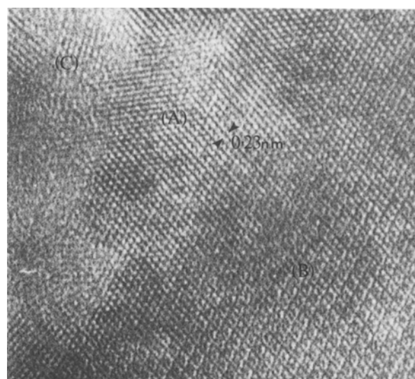
Figure 14 High resolution electron micrograph of an ordered domain obtained with the electron beam parallel to the [1 1 0] and the objective aperture enclosing both the sub-lattice and superlattice reflections. The dark fringes arise as a result of the superposition of \{1/2\ 1/2\ 1/2\} superlattice reflections onto every second \{111\} reflection.
